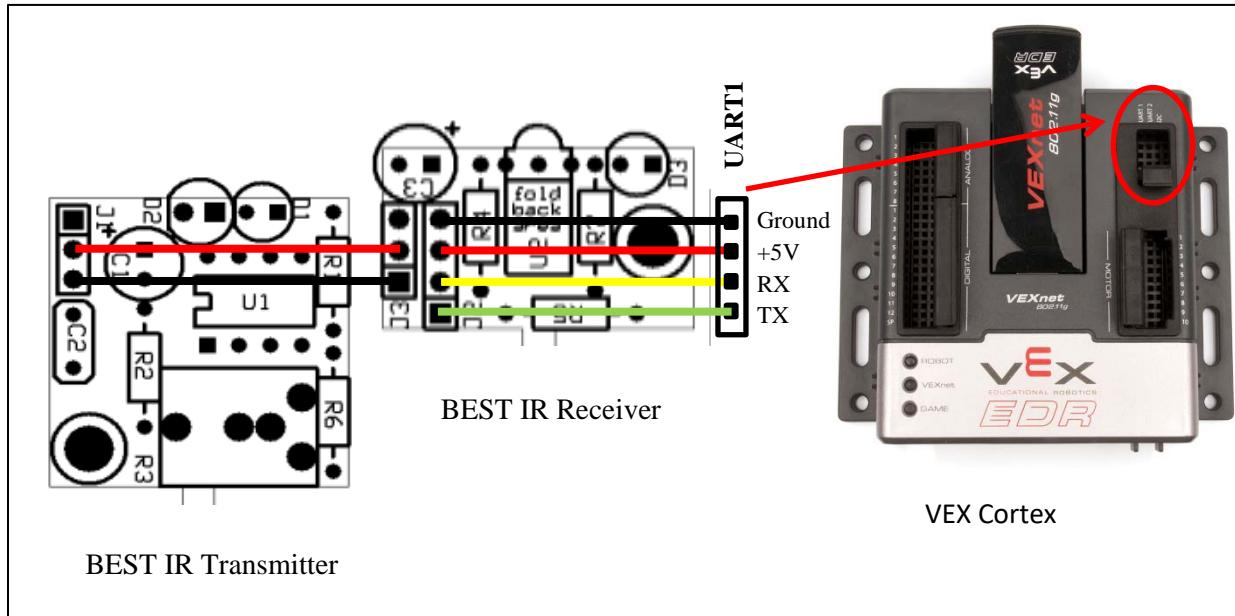
Ideally this hookup would use a 4-wire M-F cable and a 2-wire M-F cable. Since we don't have those in the kit you will need to improvise. A servo extension cable plus a single wire will work to connect the receiver to the Cortex. The IR transmitter connects to the IR receiver using only 2 wires, so *don't* use a servo extension cable for this connection.
