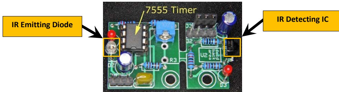
The board that emits the IR light is the transmitter and is the larger of the two boards. The IR emitting diode is the clear one, located on one edge of the board. Note that as supplied it emits light in a direction perpendicular to the plane of the board. If you want it to emit light in the plane of the board, **carefully** bend the two leads 90 degrees, the IR diode will extend beyond the edge of the board.
