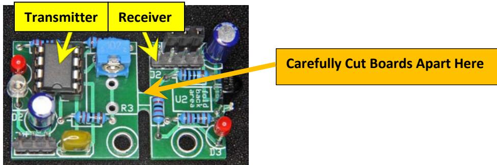
In the kit the two PC boards are manufactured as a single board to make it a little larger for easier assembly. After soldering on all the components, the two boards will be cut apart. If you have not already done so, cut the board as described in the final step of the assembly instructions.
