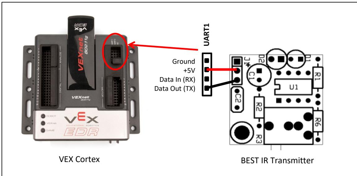
Yes, the Cortex TX pin drives the BEST IR transmitter ground pin. The IR transmitter board acts as a single component that emits IR pulses as long as Cortex Data Out pin is pulled low.
