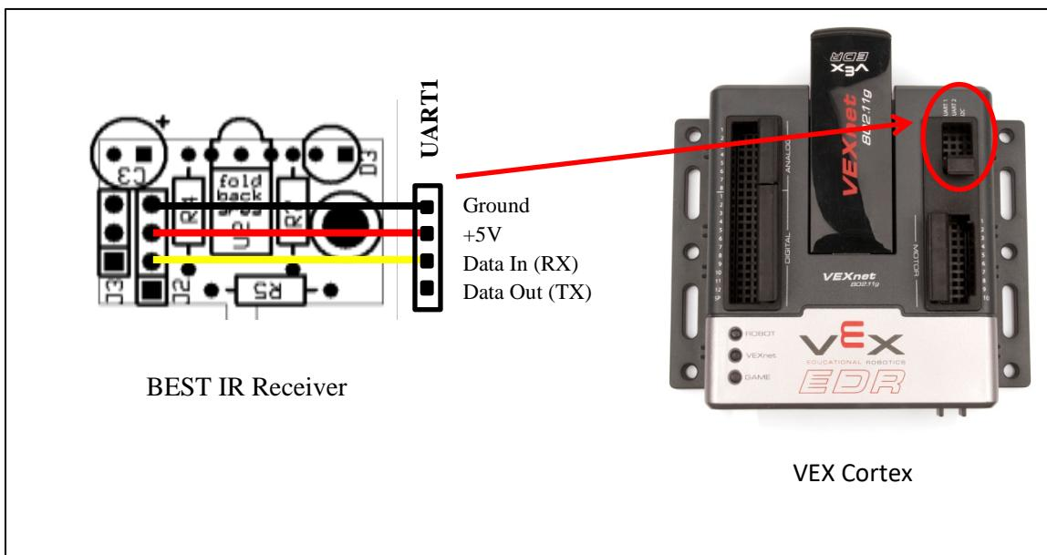
Using a 3-wire M-F servo extension cable, connect the receiver board to the Cortex as shown above. Make sure you don't end up with a twist in the cable.
